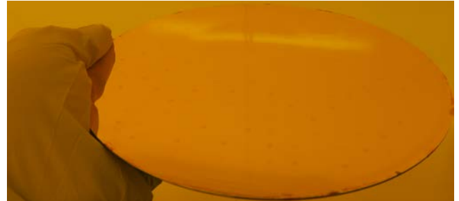
Figure 8: 200 mm wafer after copper plating
