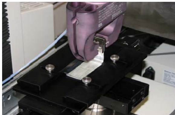
Figure 3: Tape is peeled at a 90° uniform pull from the substrate
