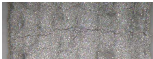
Fig. 13. Cracks appeared in the SF antenna after 1000 bending cycles (mag. 100 X).
