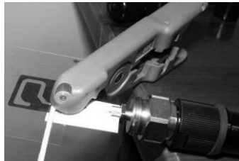
Fig. 7. A probe used in performed return loss measurements.
