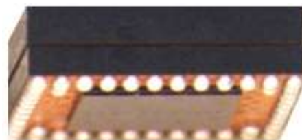
Figure 9 - Final WL3D / WLPoP-1 configuration with 3 levels of functionality (2x eWLB based WLSiP stacked, and 1x “Hanging Die” Flip-Chip assembled in ball grid array)
