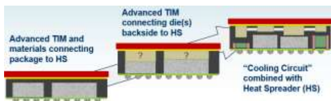
Figure 12 - Advanced thermal performance improvement solutions for eWLB based WLSiP of increasing complexity
