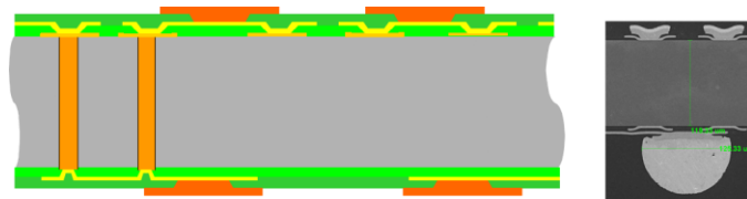
Fig. 8: Schematic of silicon interposer with TSVs (left) and actual cross-section (right)
