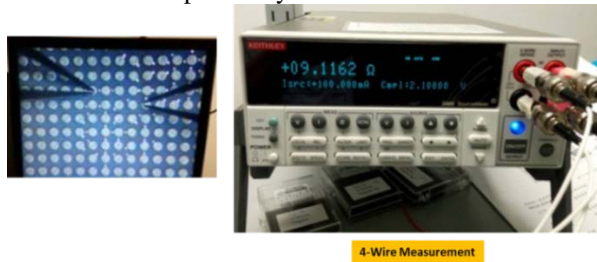
Figure 10 the measurement of daisy chain resistance for SiP.
