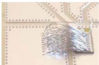
Fig. 5. Silver sintered die attach with 125 \mu\text{m} aluminium multi wire bonds [6]
