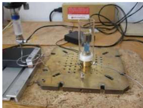
Fig. 8 Real experimental combustor (centre) with flowmeter and syringe pump (both on the left).
