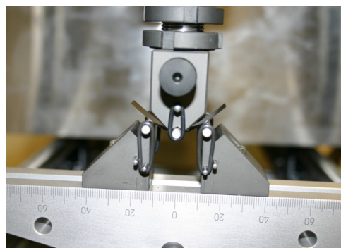
Figure 4. A bend test in progress.
