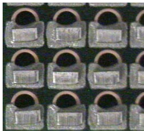
**Figure 10.** Solder paste is printed and the preforms are placed on the paste as shown.
