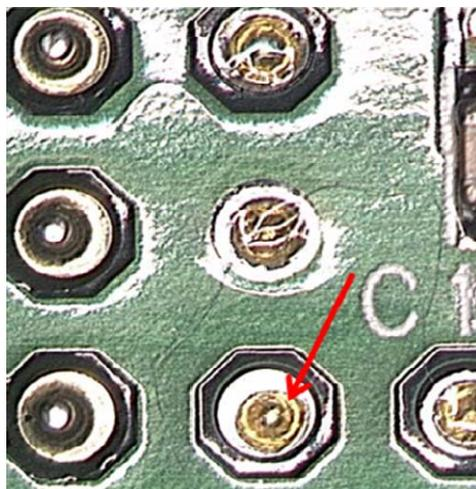
**Figure 7.** The arrow points to a pin soldered with the PIP process. Note the excess flux.
