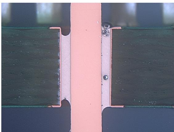
**Figure 8.** Note the lack of solder in this PIP through-hole solder joint.
