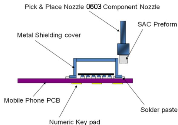
**Figure 13.** The SAC preform is placed by the component placement machine in the location.
