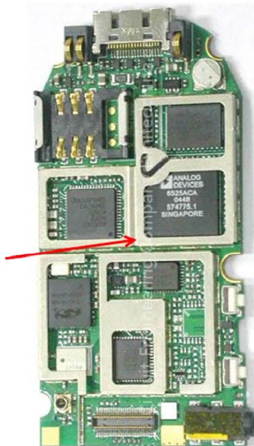
**Figure 12.** A mobile phone PCB showing a Faraday shield. Many shields are not cut away as these are. Photo courtesy of China Telecon.
