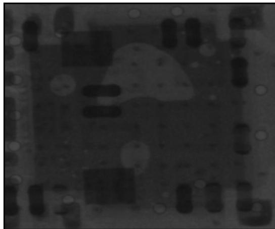
**Figure 3.** An X-ray image of the voiding between the QFN thermal pad and the PWB
