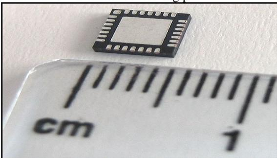
**Figure 2.** A QFN showing its leads and thermal pad for the QFN thermal pad.
