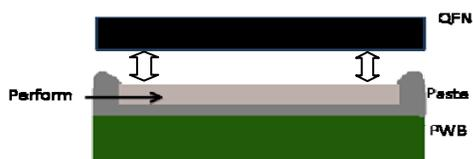
**Figure 4.** A rectangular solder preform placed on the solder paste.
