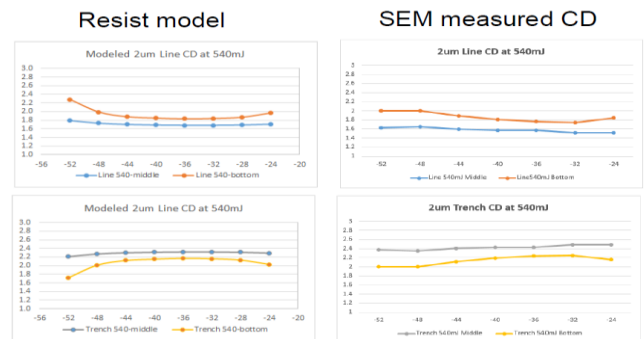
Fig. 4: Photoresist model compared to measured CDs through focus
