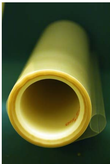
Figure 6. BCB laminate dielectric on plastic core
