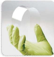
Fig. 5. Manufacture of high quality ultra-slim flexible Willow™ glass provides substantial opportunities to deliver substrates for TGV that do not require post processing.
