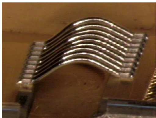
Figure 1(a) 10 mils aluminum wires bonded on gold plated submount at room temperature
