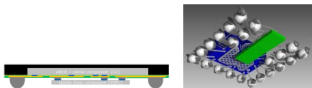
Fig. 12. (left) Scheme of two dice face to face in an eWLB; (right) X-ray tomography image of the two dice face to face in eWLB.
