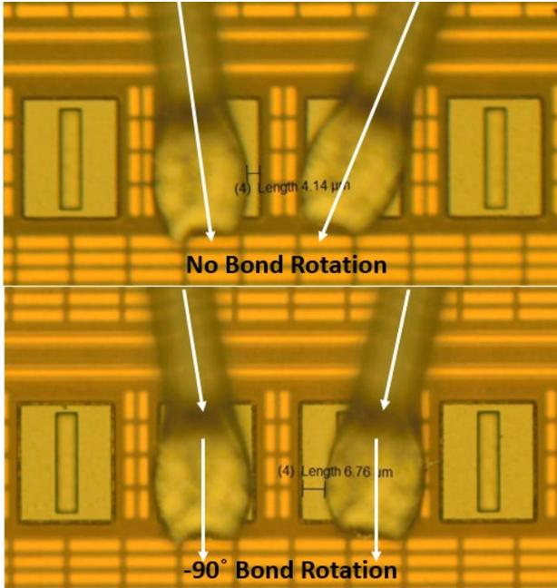
Figure 5: Bond rotation effects on bond placement
