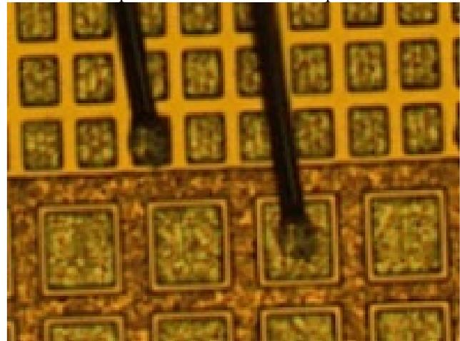
Figure 2: 0.7mil wire bonded to  $30 \mu\text{m} \times 37 \mu\text{m}$  pads (left) and  $53 \times 60 \mu\text{m}$  pads (right)
