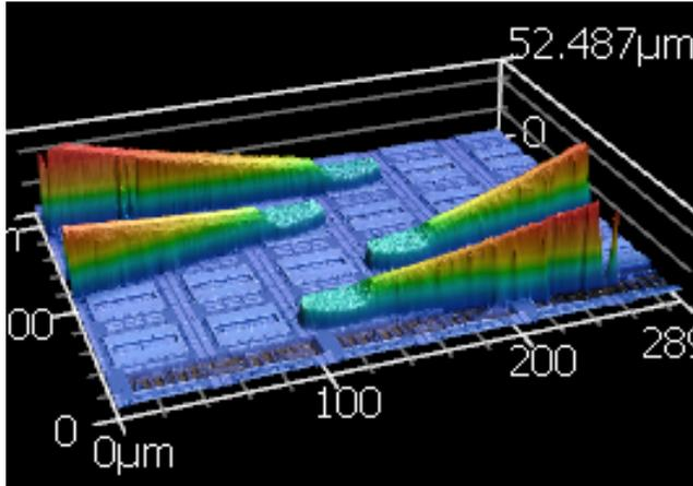
Figure 3: 3D image of wires from Fig. 1 (Keyence VK-X1000)
