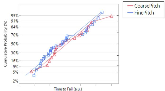
Figure 7: Reliability Stress Results between 0.7mil Al, 43 μm pitch test structures (blue) and 1mil Al, 86 μm pitch test structures (red).
