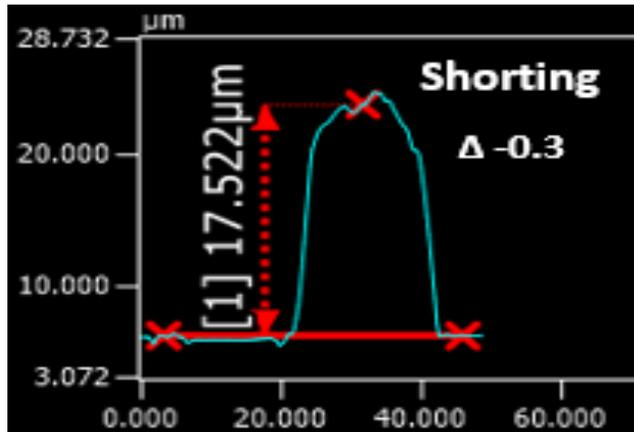
Figure 4: Wire distance above shorting pad confirms shorting (Keyence VK-X1000)
