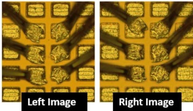
Figure 6: Bond placement repeatability with high material placement variability
