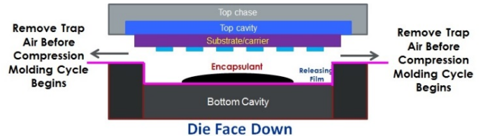
Fig. 10: Evacuation of Air Trap Before Compression Molding Cycle
