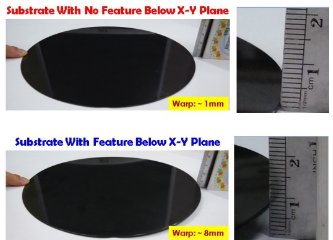
Fig. 15: Warpage Comparison No Trench vs. Trench Silicone Wafer [3]
